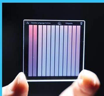
Introducing nanostructures into fused quartz using a femtosecond laser leads to a 5D memory crystal that remains stable for 1,000 years. The sample shown here archives 13,000 pages written in 1,500 human languages (2 columns, 4 GB) and Wikipedia text from 2020 (10 columns, 24 GB)
