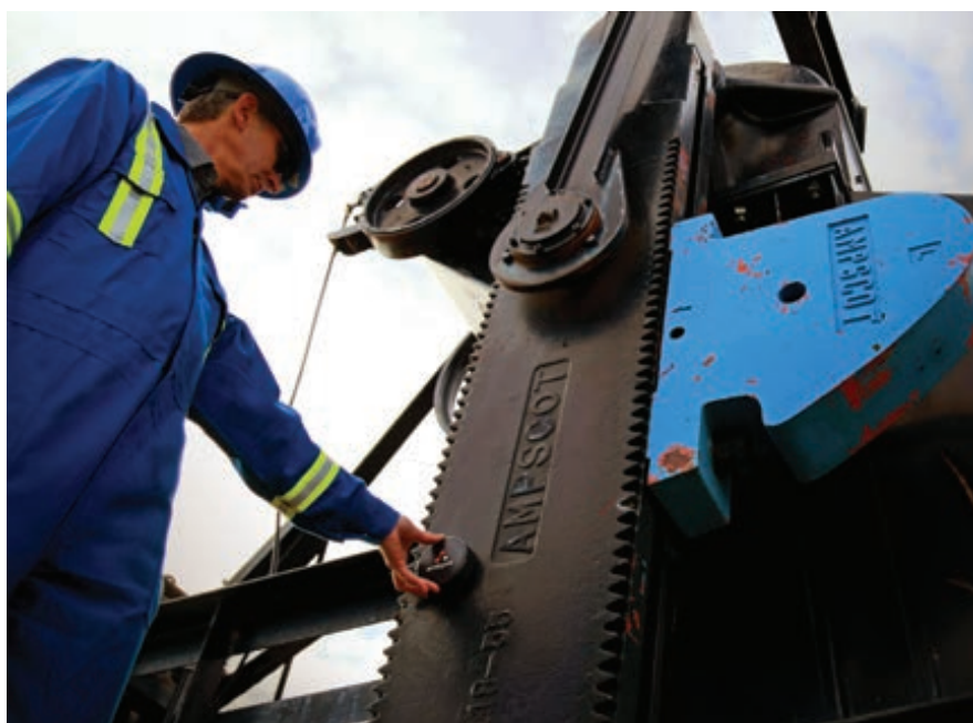
A worker installs a small sensor on a pump jack which turns the machine into an internet-of-things device that can be tracked, monitored, and controlled remotely or set to optimize itself autonomously. Source: Ambyint
